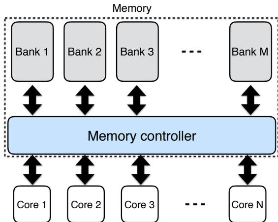
Fig. 1: Multi-core Architecture with shared memory.
