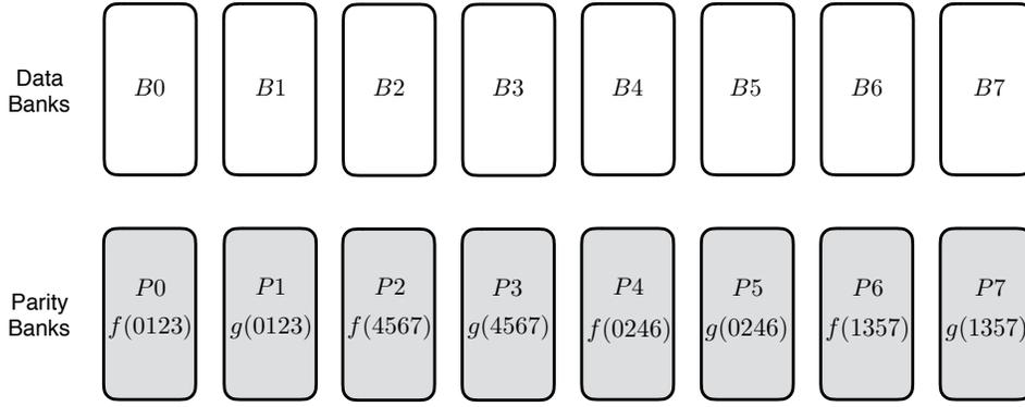
Fig. 6: Data storage layout for coded memory system
