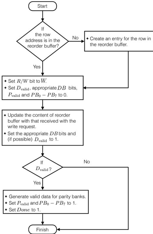
Fig. 8: Description of the write algorithm.
