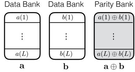
Fig. 2: Parity bank obtained by performing bit-wise XOR on the two data banks  $\mathbf{a}$  and  $\mathbf{b}$ .
