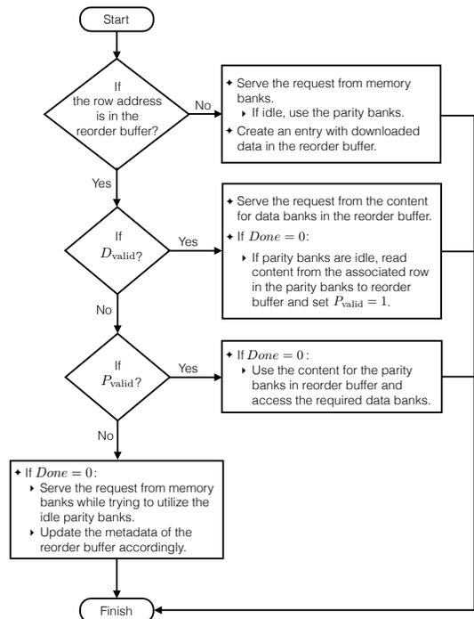
Fig. 7: Description of the read algorithm.
