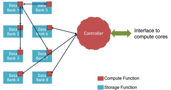
Fig. 5: Block diagram description of new memory system architectures with distributed memory controllers. This architecture includes a control logic closer to the data bank. This control logic is capable of certain fixed computation that can be exploited to reduce the access bandwidth between the bank and the main controller.
