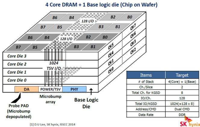
Fig. 4: High Density Memory (HBM) architecture<sup>2</sup>. The 3D stacking of memory channels provides an orthogonal plane to pack a large amount of storage in a smaller footprint while maintaining the system’s electromagnetic characteristics.
